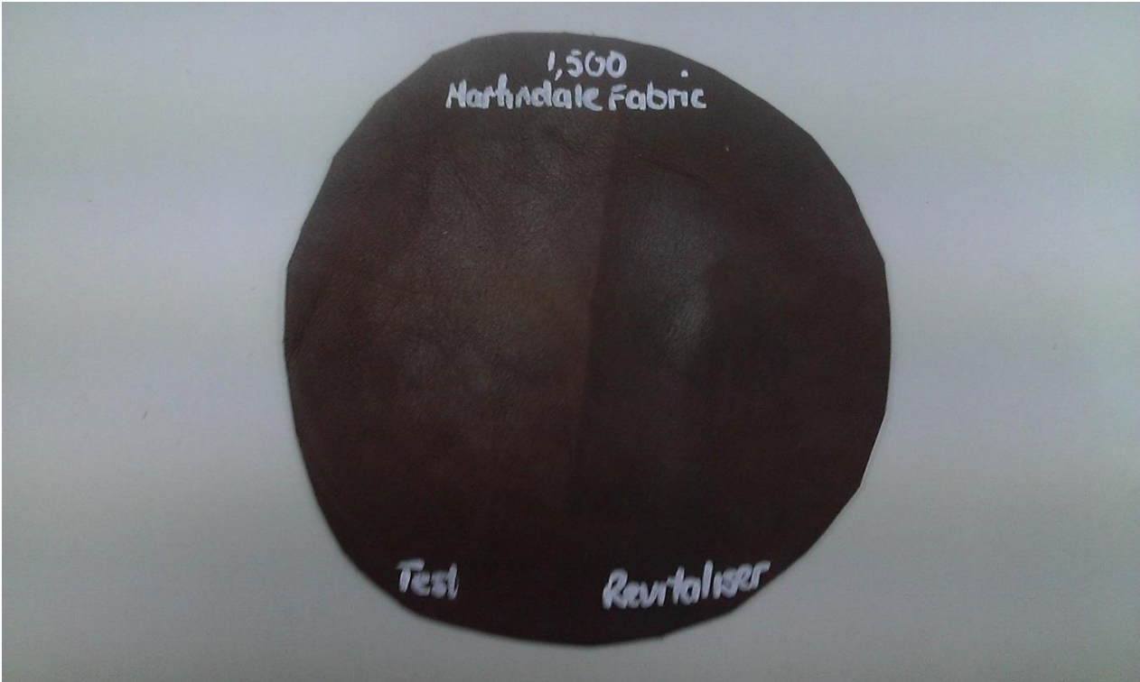
Figure 9: Damaged leather sample showing damage on left side and near complete restoration on right side after revitaliser is applied.
