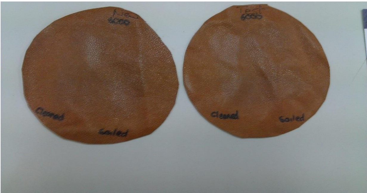
Figure 3: The photographs above show the semi aniline leather after 6,000 soiling cycles. The untreated leather is on the left, and the protector treated leather is on the right.
