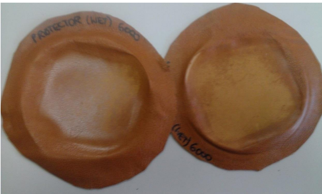
Figure 7: Sample on left - Conditioner/Protector treated leather. Sample on right: Untreated leather
