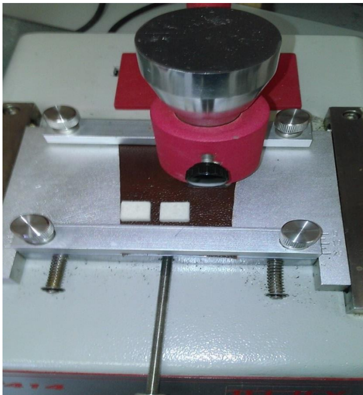
Figure 2: The rub fastness test arrangement is shown above.
