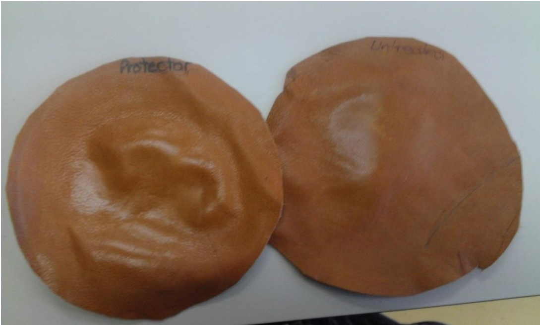
Figure 6: The left sample is treated with conditioner/protector and withstood 2,500 cycles on the Martindale abrasion tester, whilst the sample to the right is untreated and shows finish damage after just 500 Martindale abrasion cycles
